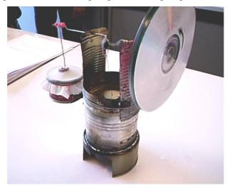
A Stirling engine gamma type is easy to build with cans.
